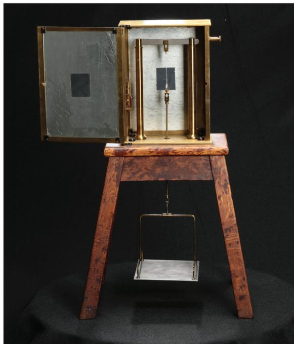
This is one of two original piezo machines that the Curies employed in their discovery of radium and polonium. As a forerunner to the modern dosimeter, it was one of the first tools to measure radioactivity. After years of use in the Curie laboratory, Marie Curie donated the device to The College of Physicians of Philadelphia on a visit in 1921.
